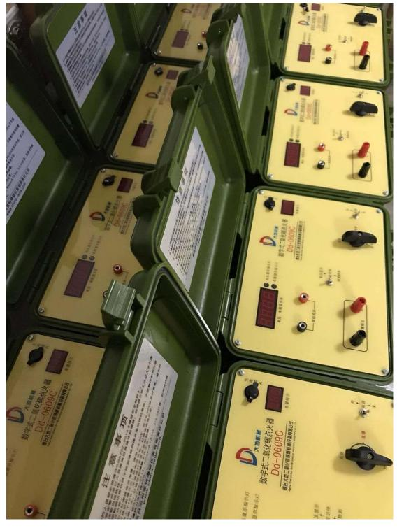
Figure 4 Digital carbon dioxide igniter
