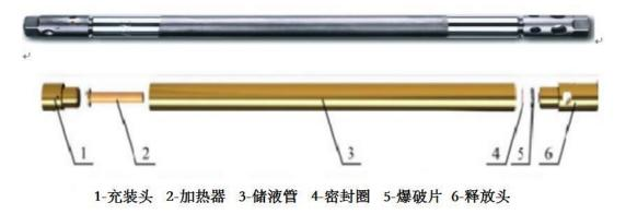
Figure 3 Schematic diagram of carbon dioxide expansion tube structure 充装头 Filling head 加热器 Heater 储液管 Liquid storage tube 密封圈 Seal ring 爆破 片 Blasting piece 释放头 Moving head
