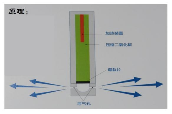
Figure 1: Schematic diagram of intelligent carbon dioxide cracking system 加热装置: Heating device 压缩 CO<sub>2</sub>: Compressed CO<sub>2</sub> 爆裂片 bursting piece 泄气孔: air leakage hole
